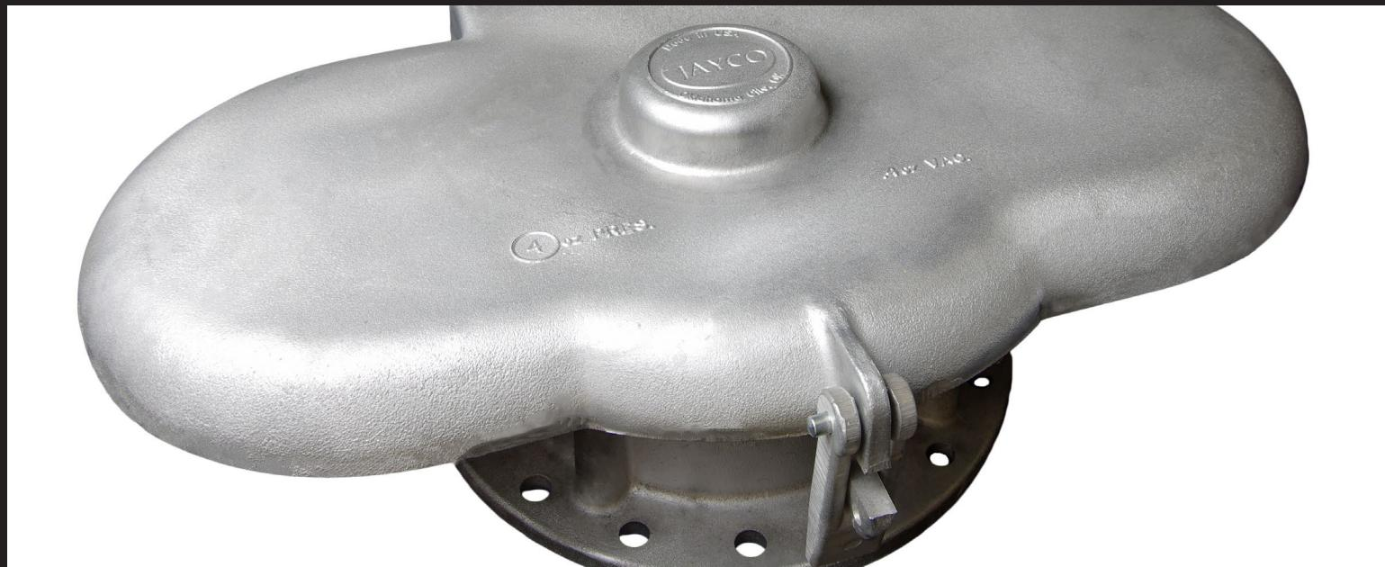
THE PURPOSE OF THE THIEF HATCH IS TO WORK IN TANDEM WITH THE VENT VALVE TO MINIMIZE THE ESCAPE OF LIGHT ENDS OF CRUDE IN LEASE STORAGE BY MAINTAINING A PRESSURE ON THE TANK. A VACUUM RELIEF FUNCTION IS ALSO STANDARD. THE THIEF HATCH PERMITS ACCESS TO THE CONTENTS OF THE TANK FOR SAMPLING AND GAUGING. THE JT-20.2 FEATURES A 20" OBLONG DRIP PAN TO CONTAIN DRIPPINGS AND GIVES THE OPERATOR A WORKSPACE FOR TOOLS.
