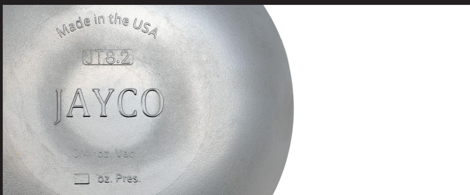
THE PURPOSE OF THE THIEF HATCH IS TO WORK IN TANDEM WITH THE VENT VALVE TO MINIMIZE THE ESCAPE OF LIGHT ENDS OF CRUDE IN LEASE STORAGE BY MAINTAINING A PRESSURE ON THE TANK. A VACUUM RELIEF FUNCTION IS ALSO STANDARD. THE THIEF HATCH PERMITS ACCESS TO THE CONTENTS OF THE TANK FOR SAMPLING AND GAUGING. THE VENT VALVE SHOULD BE SET TO VENT PRESSURE BEFORE THE THIEF HATCH.
