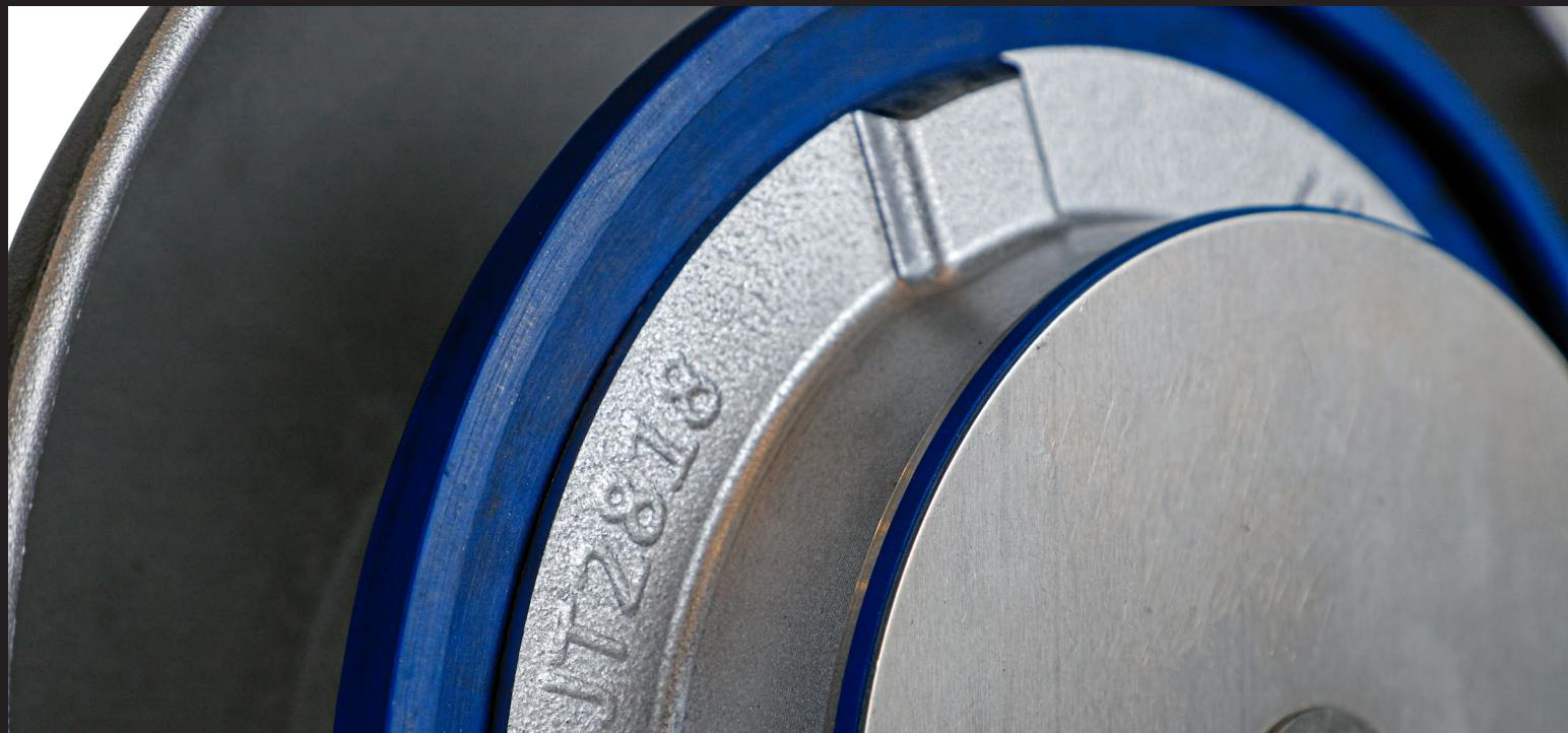
JAYCO BLUE VITON® GASKETS ARE PREMIUM MOLDED GASKETS. ON THE JT-8.2, THE PRESSURE GASKET IS PLACED IN A DOWNWARD ORIENTATION TO ASSIST IN CENTERING THE PLUNGER ASSEMBLY, AID IN PLUNGER LIFT DURING VENTING, & PROVIDE A DUST SHIELD FOR THE SEALING SURFACE. THESE ARE EASILY IDENTIFIED AS VITON® BY THEIR RICH BLUE COLOR.
