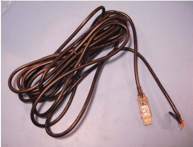
Figure 10 - FTDI Chip USB-RS485-WE-5000-BT, 5m, USB to RS-485 Cable
