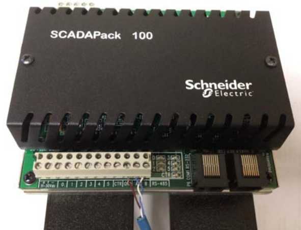
Figure 21 - SCADAPack 100 With Attached CAT5E Cable
