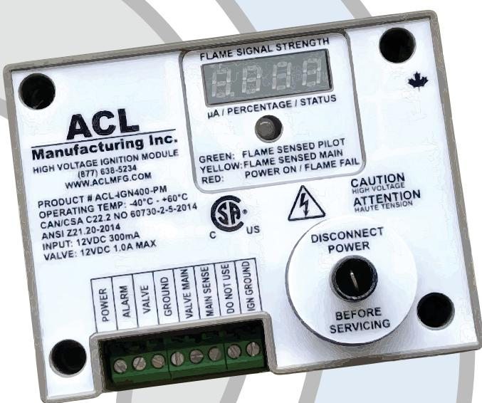
The **ACL IGN400-PM Ignition Module** is designed to light and monitor a pilot, reacting quickly to a loss of flame and acting to relight the pilot. It uses a single flame rod for both Ignition and Flame sensing, displaying the flame signal strength on the display and with LED indication. The Ignition Module can also monitor a main flame using a second Ignitor rod.
